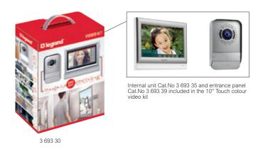
2-wire colour video hands-free kit with surface mounting street panel (with rainshield included). Kit can be expanded up to 2 apartments. In each apartment it is possible to manage up to 3 internal units
